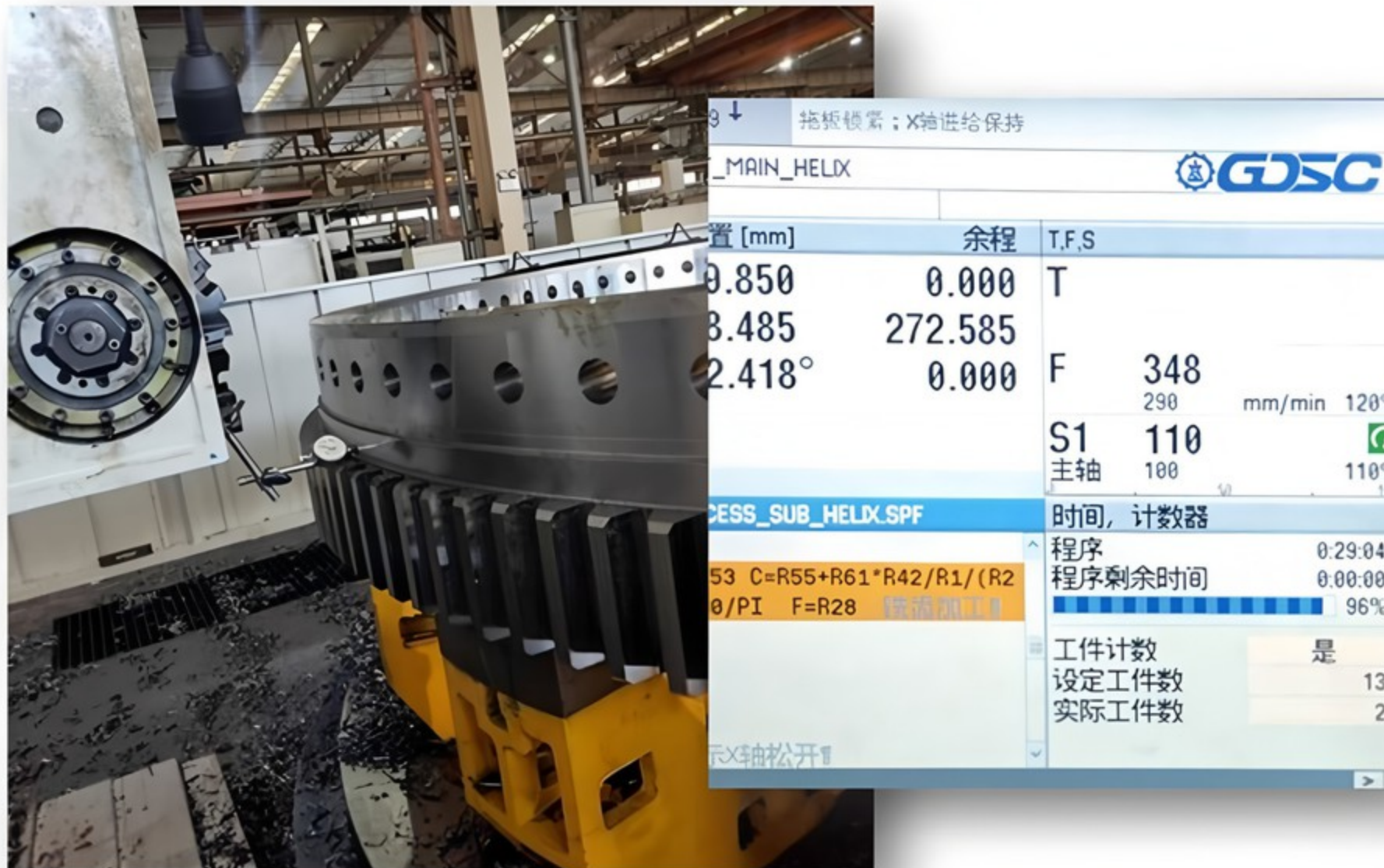
M24 Z139 External gear finish milling operation and parameters
